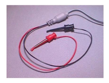
Figure 1. The Voltage Sensor
