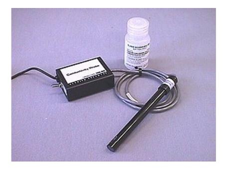
Figure 1. The Conductivity Sensor
