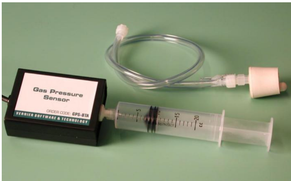
Figure 1. The Gas Pressure Sensor
