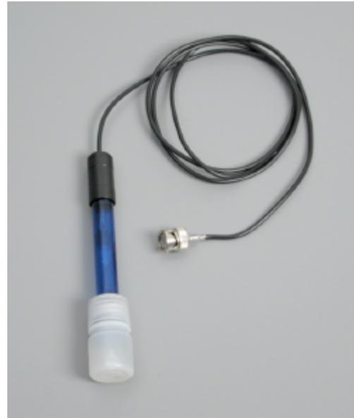
**Figure 2.** The pH electrode.
