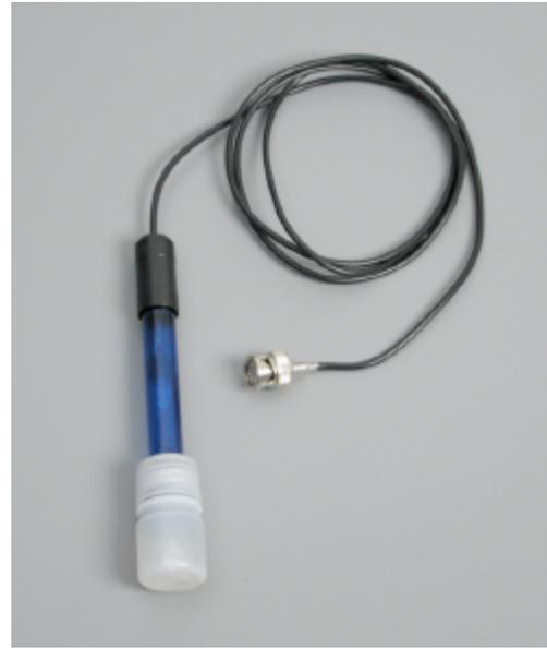
**Figure 2.** The pH electrode.
