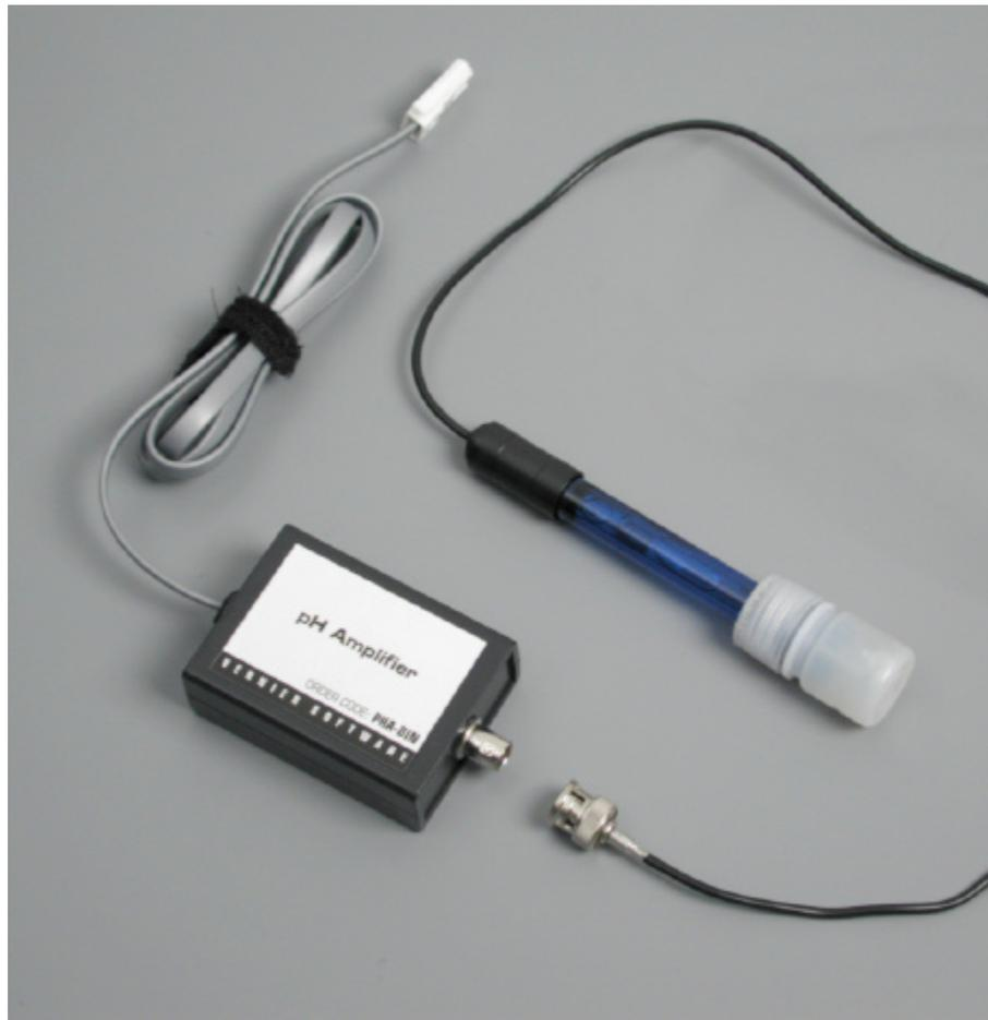
**Figure 1.** The pH System (Amplifier and Electrode)
