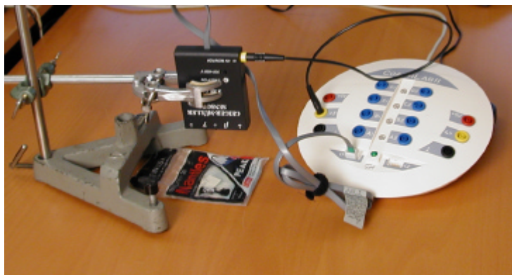
Figure 1. Experimental set-up with the CoachLab II interface. The BT connector of the GM sensor is connected to Input 1; the 4-mm connector is connected to Input 3.
