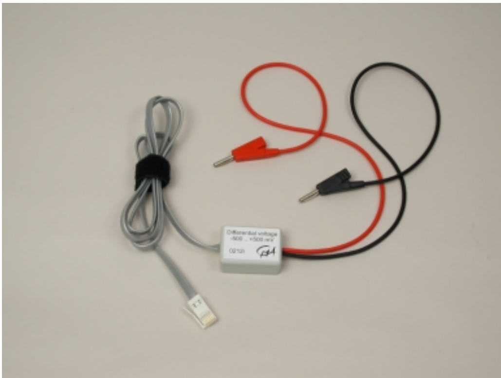
Figure 1. The Differential Voltage Sensor - 500 .. +500 mV
